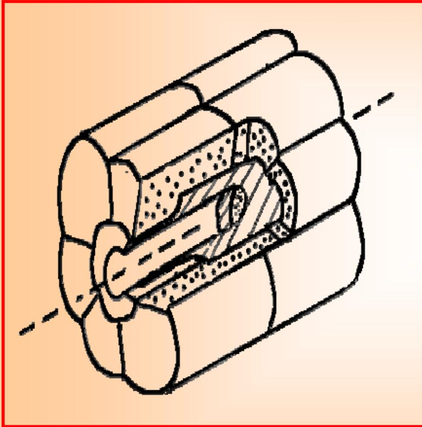
$4\pi$  - multidetector system ROMASHKA (Daisy) for gamma low activity measurements is assembled from 12 scintillators NaI(Tl) which are divided on two halves of 6 crystals with a special shape (like a flower Daisy). The crystals measure in total are 16.6 l NaI(Tl) and they are placed in a cylinder with the outside diameter 30 cm
