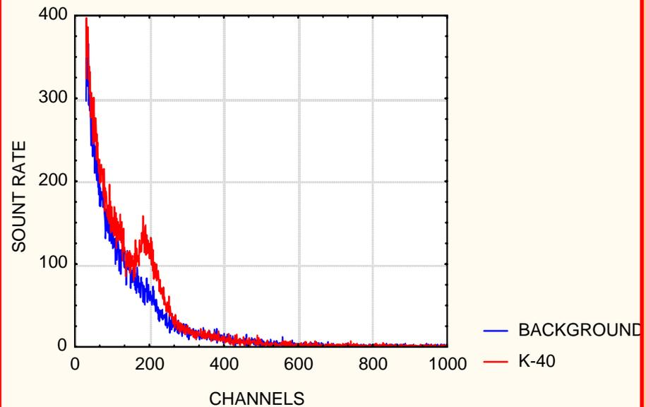
The efficiency of gamma quanta registration in this mode decreases to 40 % but it is quite enough as in this way we have the optimal ratio of efficiency and resolution. So we can recognize some peaks and group of peaks.
