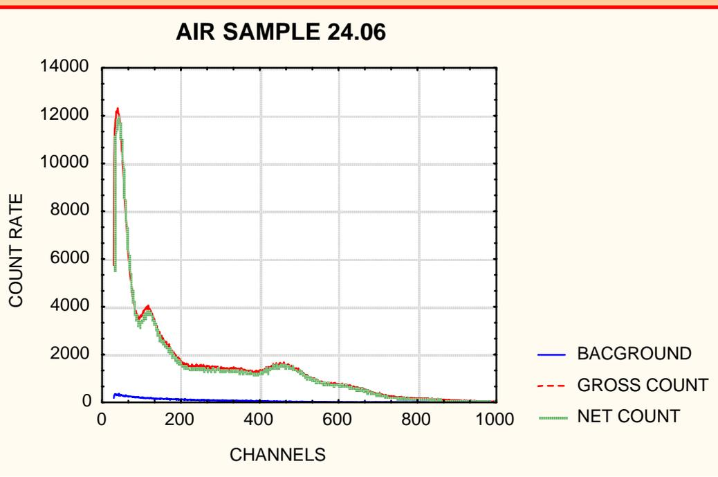
The high efficiency of registration (40 % in anticoincidence mode and 95 % usually) allows application of the  $4\pi$ -multidetector system in low activity measurements as well the improved resolution and low noise level make system suitable for samples from the environment. In anticoincidence mode of measurements we accurately estimate not only the radioactivity of the sample but also some of the radio nuclides in it.
