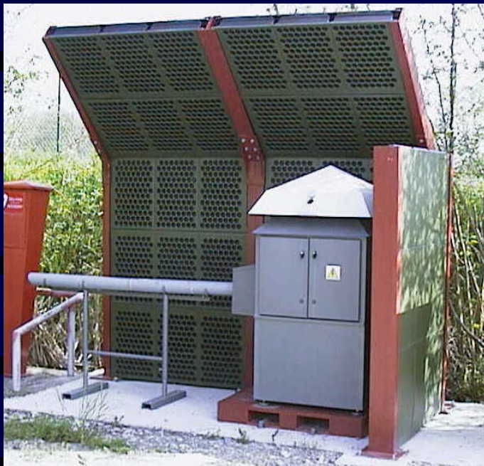
High volume aerosol sampler 600 m 3 /h
